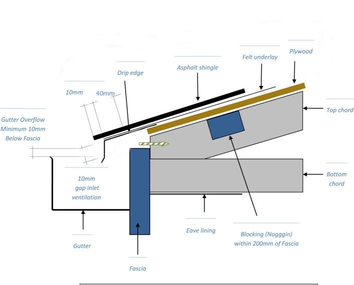
BUILDER OR ROOF FRAMER TO INSTALL NOGGIN WITHIN 200mm OF FASCIA AND WITHIN 200mm OF BOTH SIDES OF VALLEYS, RIDGES AND HIPS.
