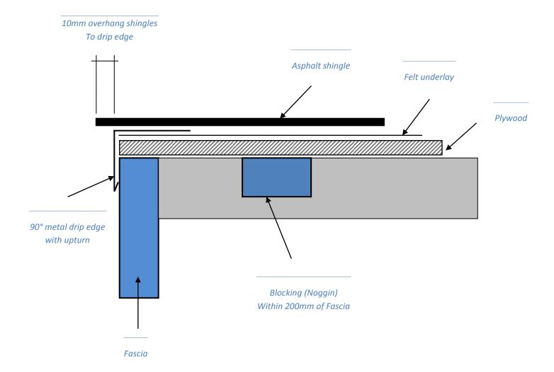
BUILDER OR ROOF FRAMER TO INSTALL NOGGIN WITHIN 200mm OF FASCIA AND WITHIN 200mm OF BOTH SIDES OF VALLEYS, HIPS AND RIDGES.
